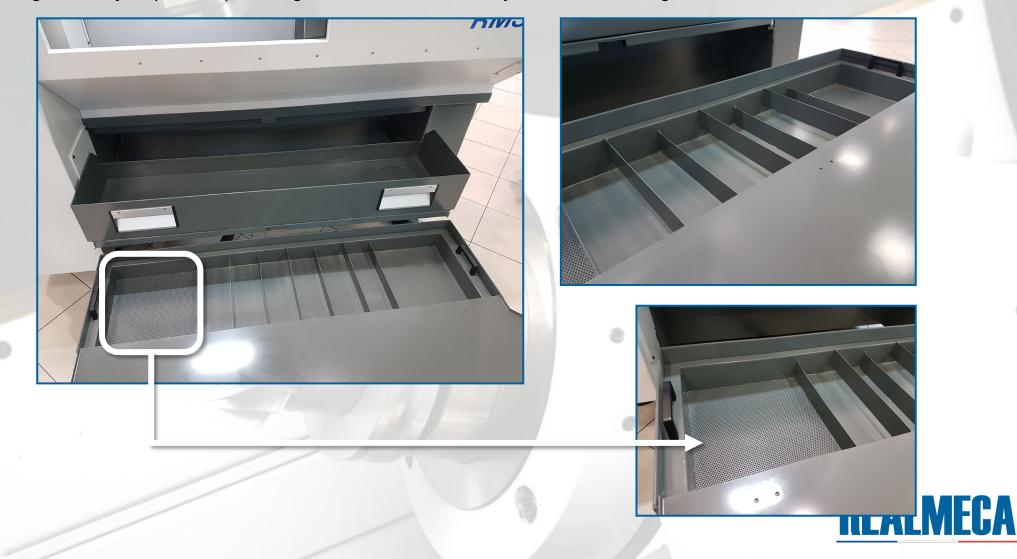
After reaching the tank at the bottom of the machine, a pump located on the left side guides the coolant through a last filter, before restarting the cycle.
