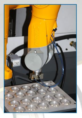
Setting up this system allows the machine to work on up to 20 parts in a row, without any action required from the operator.
