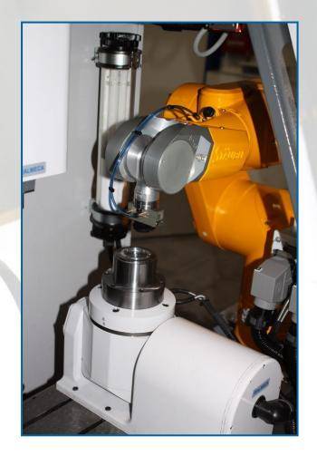
The robot arm is installed on the left side of the machine and is placed on an elevated support, attached to the machine's base.
